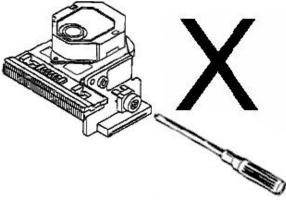
Due to the structure and operating principles of laser diode, LD may deteriorate on current surges caused by switch and high speed pulse cause by electrostatic discharge.
